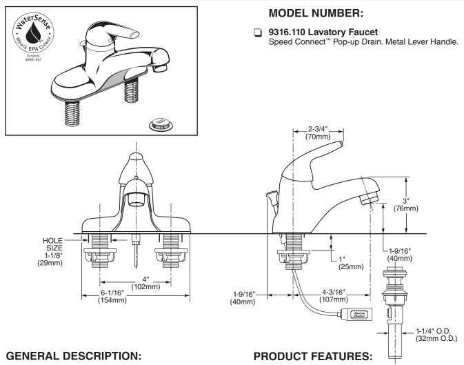
Single control lavatory faucet on 4" centers. Washerless 40mm ceramic disc valve cartridge. Durable cast brass waterway with 1/2" male threaded brass inlet shanks. Metal body with color matched underbody. Lever handle. 20" (500mm) long flexible stainless steel drain cable is pre-assembled to faucet body. Non-Metallic Speed Connect<sup>TM</sup> drain body with 1-1/4 inch (32mm) tail piece. 1.5 gpm/5.7L/min. maximum flow rate.
